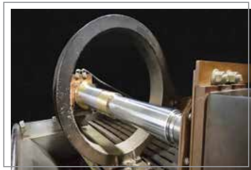
Magnetic Particle Inspection
